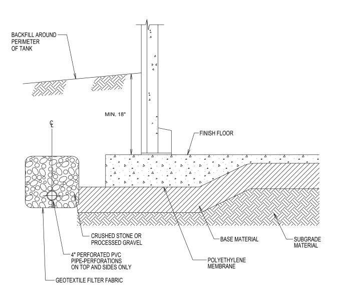
NOTE: PURPOSE OF 4" PERFORATED PIPE IS TO DETECT A TANK LEAK - PIPE TO DRAIN INTO DRAIN BOX
