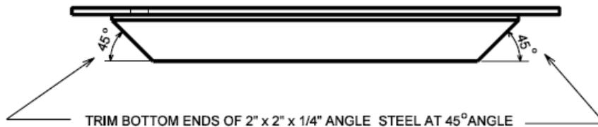
TRIM BOTTOM ENDS OF 2" x 2" x 1/4" ANGLE STEEL AT 45° ANGLE
