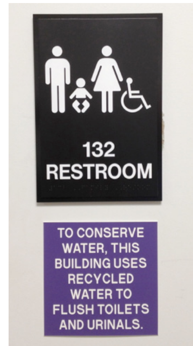
Figure 10.7 Sign at entry to bathroom using reclaimed water to flush water closet and urinals
